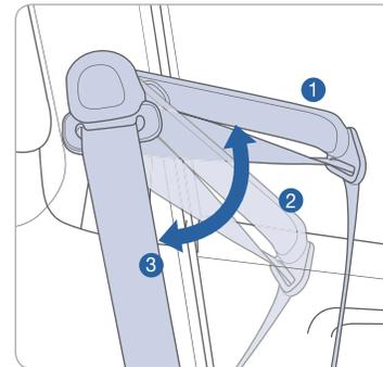
Set the belt extension guide to one of the 3 positions when using the seat belt.
