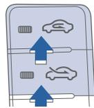
This is used to select outside (fresh) air position or recirculated air position.
