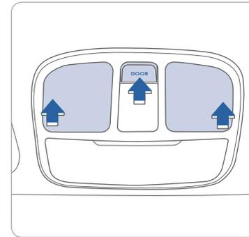
Push the switch to turn the map lamp on or off.
