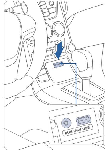
Use the jack to connect an external audio device and listen to it through the audio system in your vehicle.
