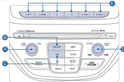
Press POWER button **A** to turn radio on.
