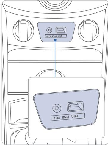
Use the jack to connect an external audio device and listen to it through the audio system speakers in your vehicle.
