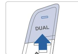
Press the DUAL button to operate the driver and passenger side temperature individually.
