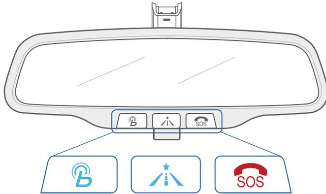
Controls for Blue Link in-vehicle voice-response use are located on the rearview mirror. (See facing page for menu of in-vehicle services.)
