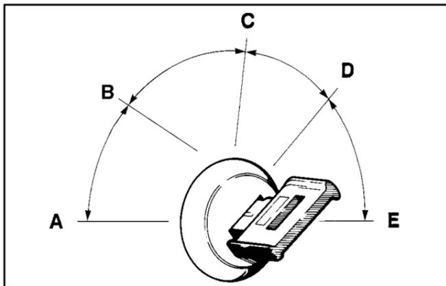
**ACCESSORY (A):** This position lets you use things like the radio, power windows and the windshield wipers when the engine is off. Push in the key and turn it toward you. Your steering wheel will remain locked, just as it was before you inserted the key.
