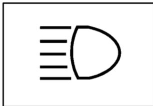
When the high beams are on, this light located on the instrument panel cluster also will be on.
