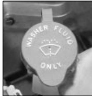
The windshield washer fluid reservoir cap is located on the driver’s side of the engine compartment. See “Engine Compartment Overview” in the Index for more information on location.
