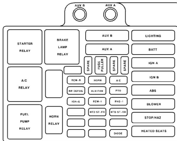
The underhood fuse/relay center is located in the rear of the engine compartment near the brake fluid reservoir. See “Engine Compartment Overview” in the Index for more information on location. Move the retainer clips for the cover to access the fuse block.
