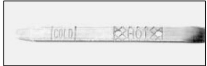
3. Check both sides of the dipstick, and read the lower level. The fluid level must be in the COLD area, below the cross-hatched area, for a cold check or in the HOT area or cross-hatched area for a hot check.
