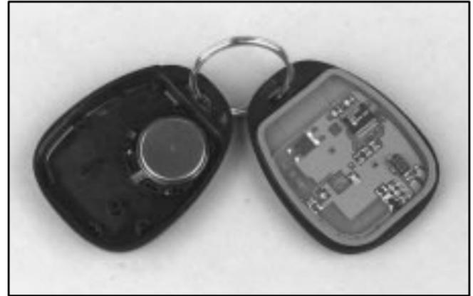
1. Insert a thin coin or flat-tip screwdriver to separate the bottom of the transmitter from the top.
