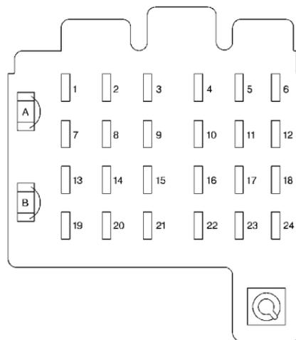
You can remove fuses with a fuse extractor which is mounted to the fuse block access door. To remove fuses if you don't have a fuse extractor, hold the end of the fuse between your thumb and index finger and pull straight out.
