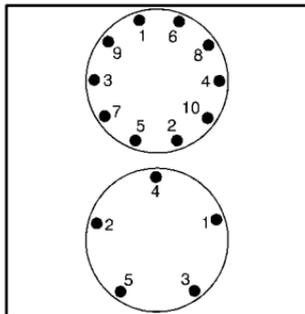
With a torque wrench, tighten the wheel nuts firmly in a crisscross sequence using the proper wheel nut torque.
