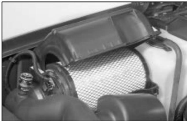
6. Install the cover and fasten the two retaining clips.
