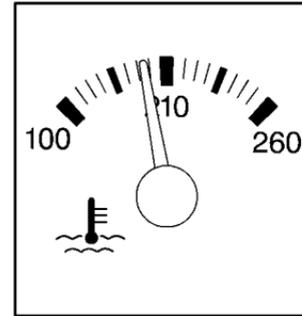
This gage shows the engine coolant temperature.
