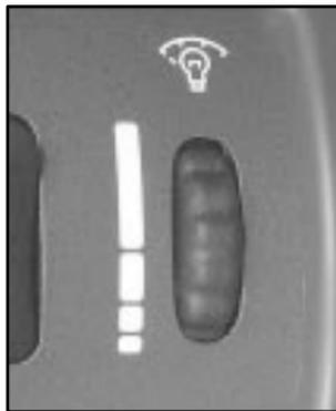
You can brighten or dim the instrument panel lights by turning the thumbwheel up or down.
