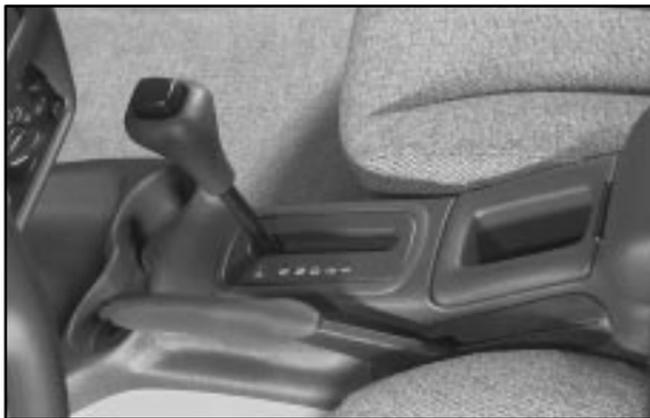
The parking brake lever is located between the bucket seats.
