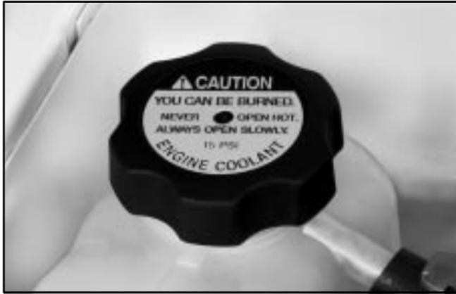
1. You can remove the coolant surge tank pressure cap when the cooling system, including the coolant surge tank pressure cap and upper radiator hose, is no longer hot. Turn the pressure cap slowly counterclockwise (left) about two or two and one-half turns. If you hear a hiss, wait for that to stop. This will allow any pressure still left to be vented out the discharge hose.
