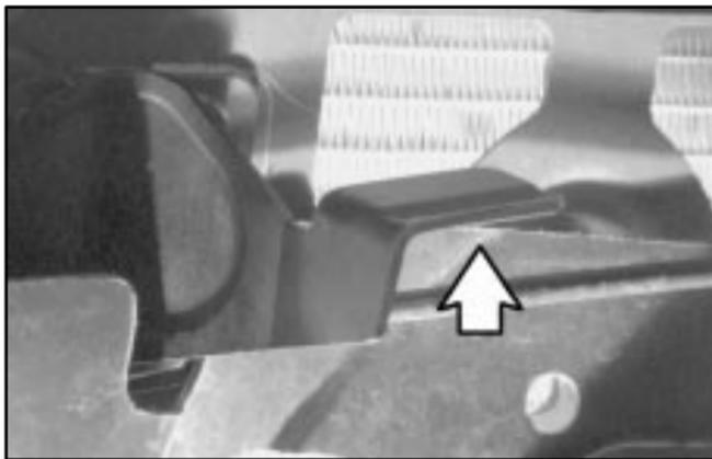
Then go to the front of the vehicle and lift up on the secondary hood release handle. The secondary hood release lever is located near the front center of the hood toward the driver's side.
