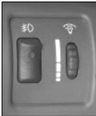
Use your fog lamps for better vision in foggy or misty conditions. The switch for your fog lamps is next to the instrument panel intensity control.
