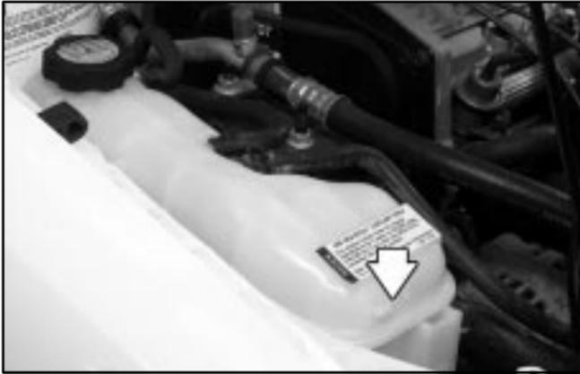
When the engine is cold, the coolant level should be at the FULL COLD mark. If it isn't, you may have a leak in the radiator hoses, heater hoses, radiator, water pump or somewhere else in the cooling system.
