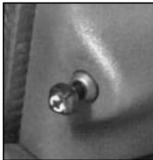
The power mirror control is located on the driver's door. Turn the control clockwise or counterclockwise to choose the mirror you want to adjust.
