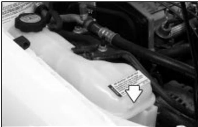
The surge tank is located on the passenger's side of the engine compartment.
