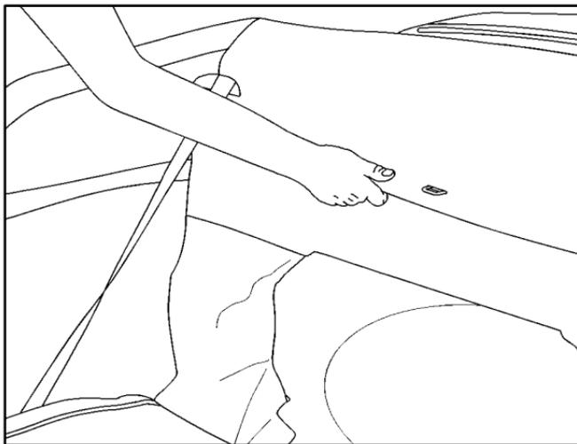
3. Gently pull the boot flap and place it over the striker which is located near the center of the rear pass-through opening.
