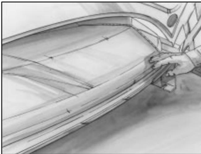
6. Go to the rear of the vehicle. Place the boot center cover along the trunk lid opening. Align one snap on the corner of the boot to the ball stud and push forward. Repeat for other snap.
