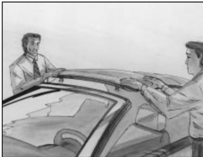
9. Pull down on the top and rotate the latch handle up to lock the convertible top. Be sure the top is latched securely on both sides.
