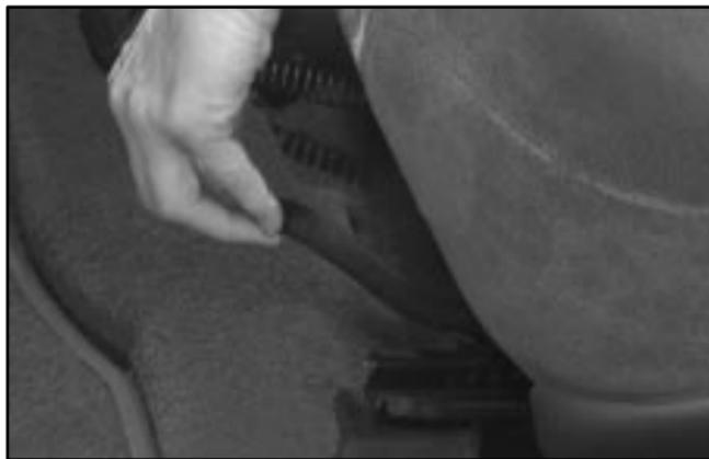
Lift the lever on the front of the driver's seat to unlock it. Slide the seat to where you want it. Then release the lever and try to move the seat with your body, to make sure the seat is locked into place.
