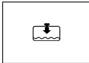
If this light comes on and stays on, your system is low on coolant and the engine may overheat.
