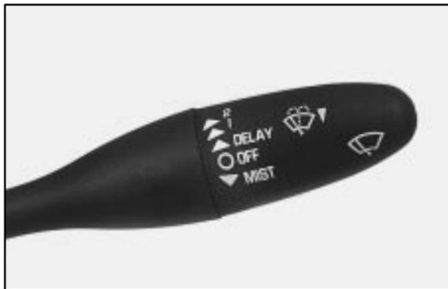
You control the windshield wipers by moving the stalk with the windshield wiper symbol on it up or down.
