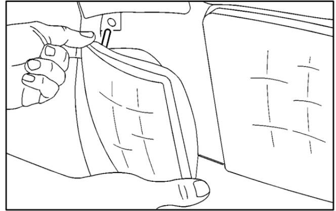
6. Push the front park and turn lamp straight in until you hear a snap. The snap feature is visible through the slot in the head lamp bracket.
