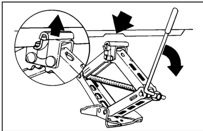
4. Raise the vehicle by turning the jack handle clockwise. Raise the vehicle far enough off the ground so there is enough room for the spare tire to fit.
