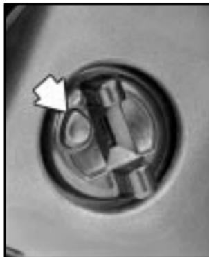
The ignition key cannot be removed from the ignition unless the key release button is used.
