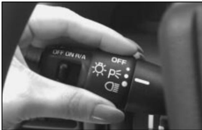
The band on the turn signal/multifunction lever controls your vehicle's lamps.
