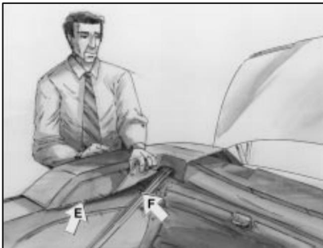
4. Attach the two snaps on the inside flap of the side cover to the top of the quarter trim panel. Attach the front snap (E) first and then the rear snap (F). The rear snap is adjustable for ease of installation. Repeat this step for the opposite side boot cover.
