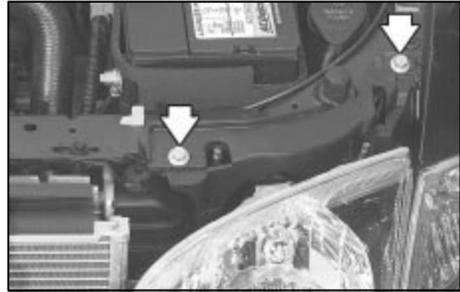
2. Using a 13 mm socket, remove the 2 bolts from the headlamp. Pull the headlamp assembly up and toward the front of the vehicle to access the bulb assembly.
