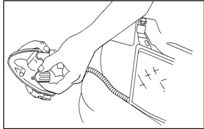
3. When the lamp is removed twist the socket to remove from the lamp. (The bulb is connected to the wire harness).
