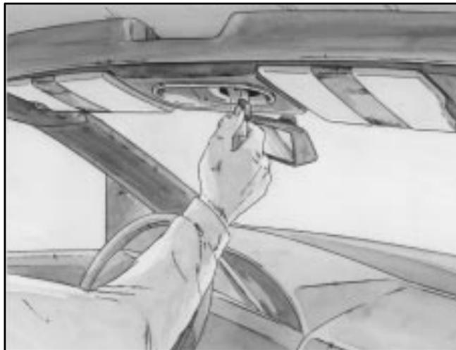
4. Push the button in the latch handle and rotate the handle down.
