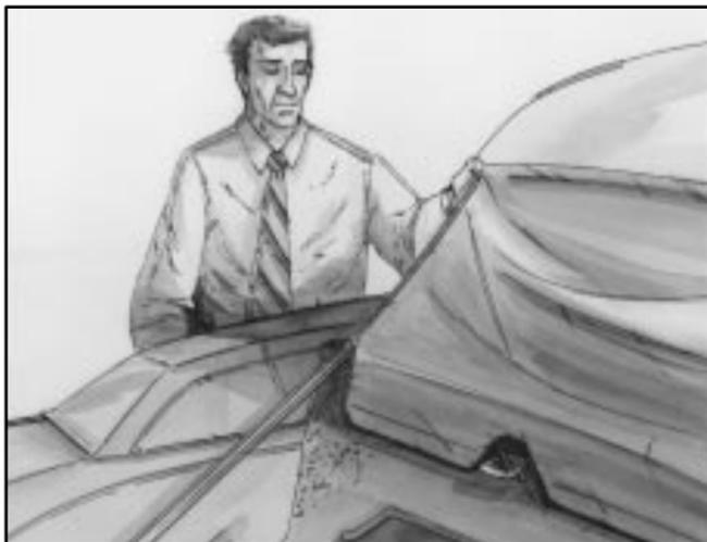
4. Go to the rear of the vehicle. Pull the snap knobs rearward to disengage the rear center cover. Carefully tuck the center boot behind the rear seatback. Make sure that the center cover is not covering the rear seatback latch. Tuck the end of the center boot rearward to keep it away from the rear seatback hinge.
