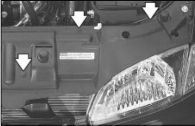
1. To remove the six plastic fasteners from the shield use the flat-head screwdriver to pull up the center of the fastener. Be careful not to break the fasteners that hold the shield in place.
