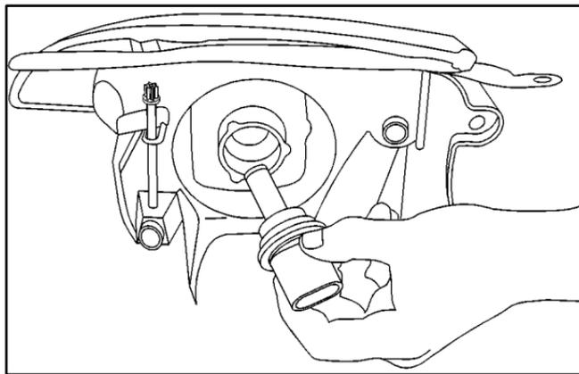
5. Remove the bulb by pulling the bulb straight out.
