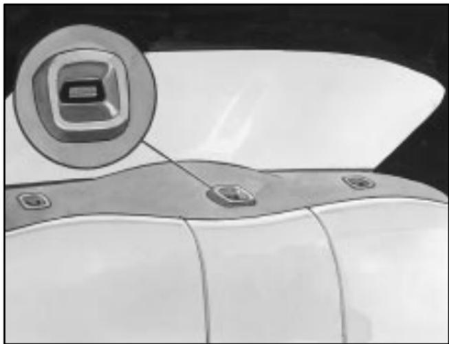
Anchor the top strap to this bracket. Once you have the top strap anchored, you'll be ready to secure the child restraint itself.
