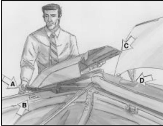
6. Lift the side cover eyelet (C) at the rear of the side boot cover from the snap ball stud (D). Raise the back of the boot side cover to unhook the tab (A) from the slot (B) in the quarter trim panel. Do the same on the other side.
