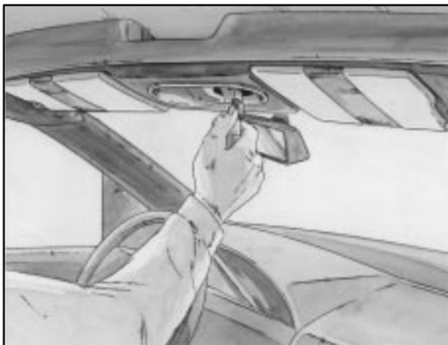
5. Pull the latch handle rearward away from the windshield and hold it until the convertible top is fully lowered.
