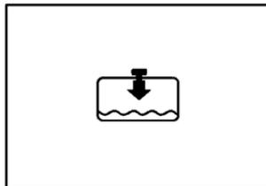
If the low coolant light comes on and stays on, it means you're low on engine coolant.
